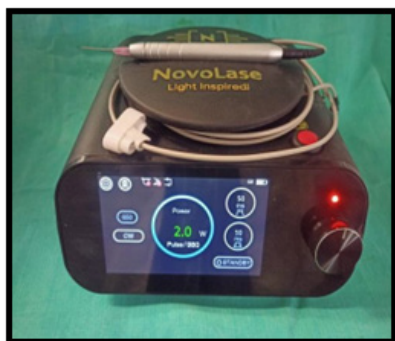
Figure 1: Diode laser: 980 wavelength, power-2 watt, continuous wave.
